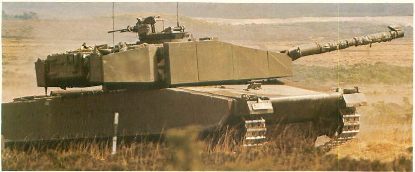
The British, French, Germans and Americans have each developed their own main battle tanks. The British Vickers VALIANT with its Chobham armour was a private venture.
